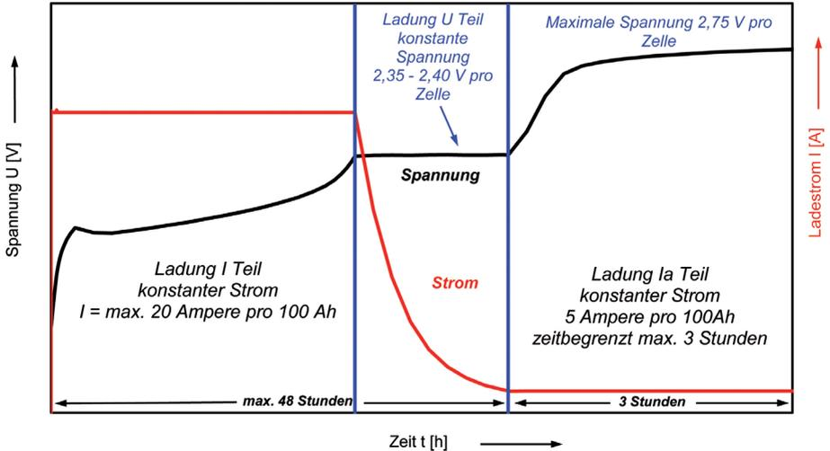
Abb. 9-2: Kennlinie IU<sub>1a</sub>
